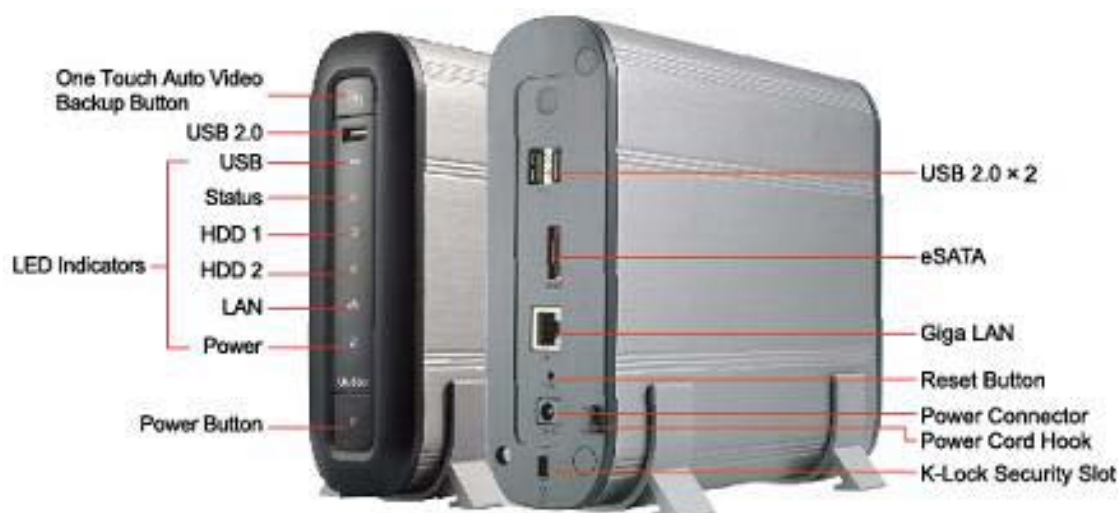
Rys.43 Serwer Q-nap Vio-Stor-101; rejestrator NVR (Network Video Recorder) oparty na systemie Linux .
